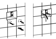
Measure the depth of the flush plate and create a cavity in the wall equal to the depth of the flush plate. Pull the pipes for installation through the cavity and thread them through the back of the base. Insert the base into the wall and Screw the fixing arms (supplied) into position. The rods may need cutting down depending on the thickness of the finished wall/surface.
